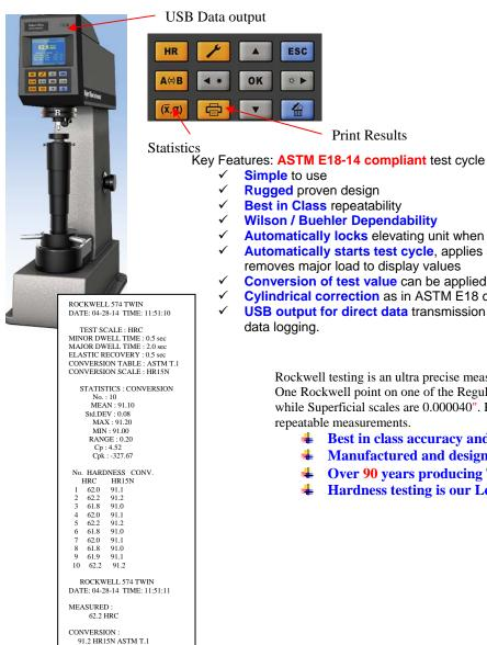
INDENTER: C Diamond MINOR LOAD: 10 kgf MAJOR LOAD: 150 kgf DWELL TIME: 2.0 sec ROCKWELL 574 TWIN Automatically locks elevating unit when mi Automatically starts test cycle, applies se
