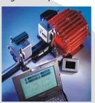
5-axis live system with color graphics and infrared communications, which eliminates the need for bulky cables and has a range of over 20 feet. The S-650 is lightweight, easy to set up and use. The S-650 uses 2 laser beams, one for angular offset, and the other for centering, making the system highly accurate. The system can
