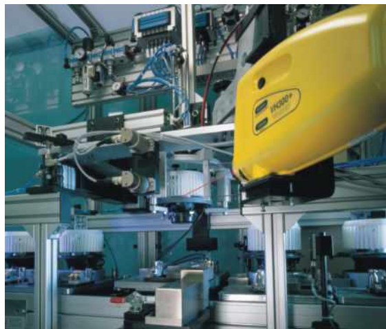
Figure 3: Test stand with laser system for noise measurement
