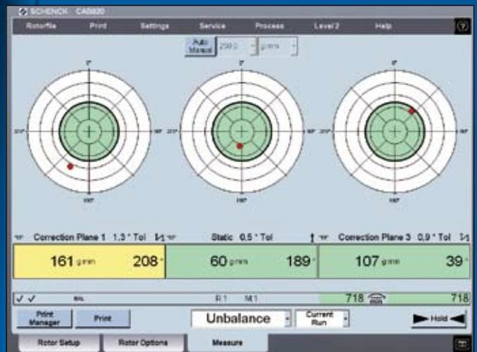
Even in the case of flexible rotors that need to be balanced in 3 planes, the operator only needs to glance at the screen to see the amount and angle of unbalance.
