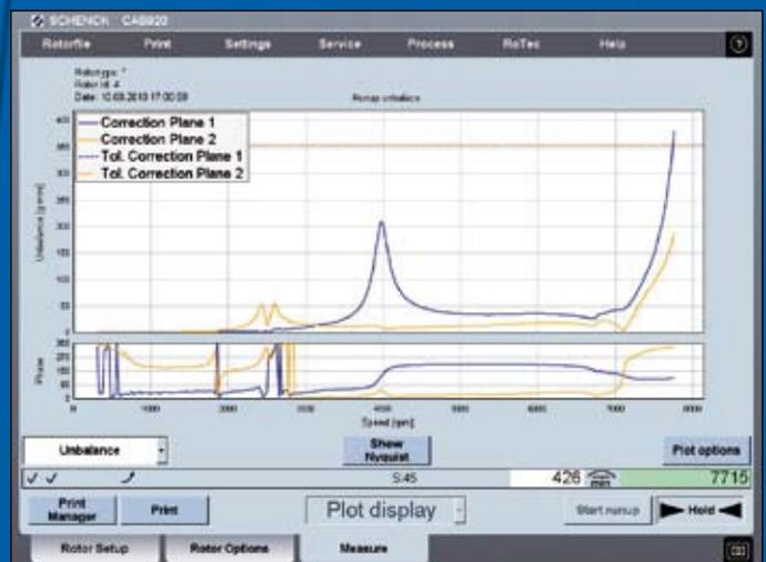
The measured values for a flexible rotor can be saved for both planes at start-up and displayed as a Bode diagram.
