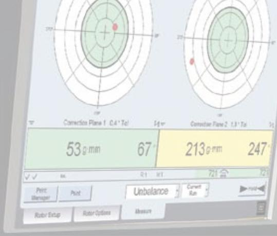
Fast and clear input of rotor data and balancing parameters is supported by the intuitive user interface.
