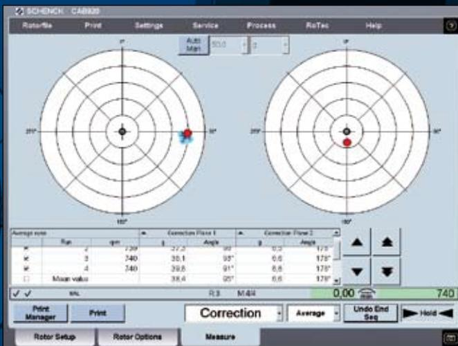
By marking the measured value and averaging over several runs, you can correct the unbalance behavior of unstable rotors.
