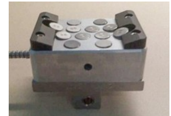
Figure 2 –Multi-Coil Eddy Current Probe
