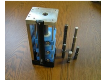
Figure 1 - Water Pump Shafts and Eddy Current Coils
