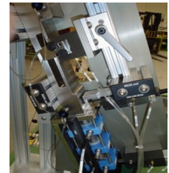
Figure 2 – In-line Sorting Station for Water Pump Shafts
