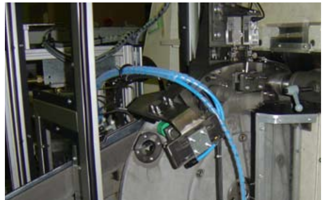
Double disc grinder type R220: detail of component clamping for gears
