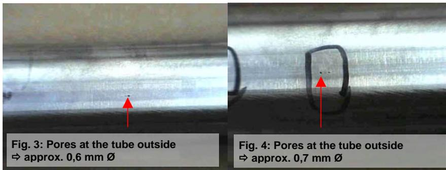
**At the tube outside the laser dropout form one or two pores; see fig. 3 and 4**
