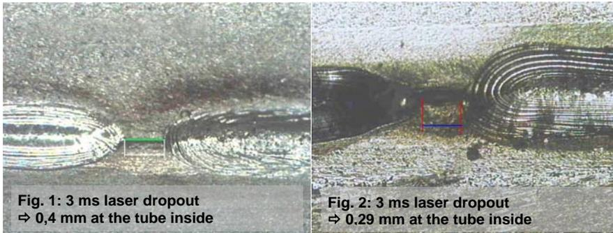
**Laser welded stainless steel tubes**
