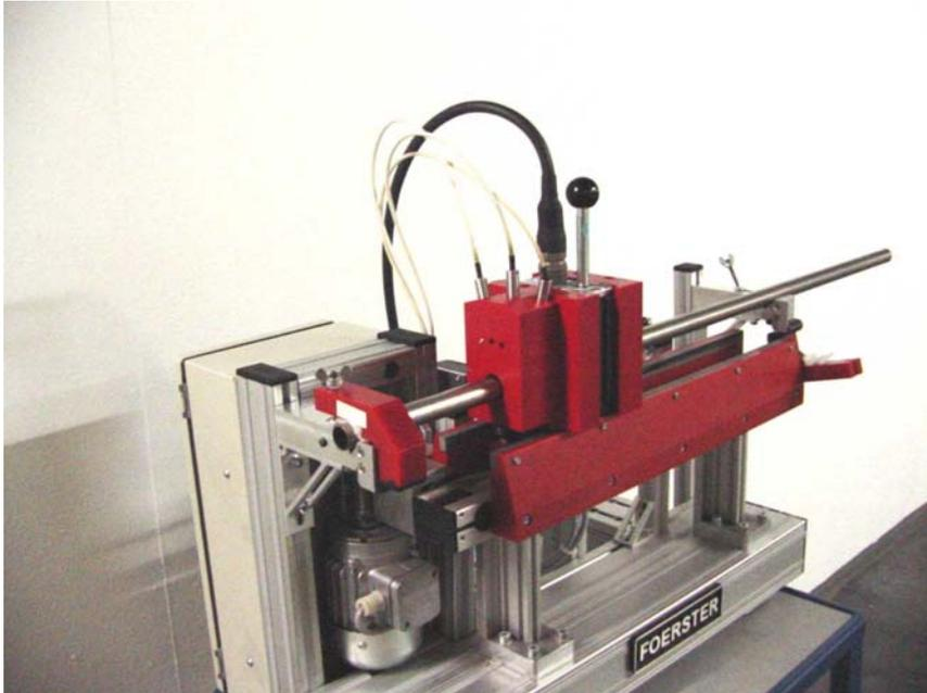
This is realised by setting up two test stations, one station equipped with a sensor array, the second station with an encircling coil. Each station works with separate signal recording up to the sorting and / or marking stage. The results of both stations are collated again for the report and for data saving.
